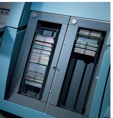
Top: The transport section is designed for high volumes and speed. The integrated NotaScan InOne Sensor provides all the security and reliability that commercial cash centers need to operate, and to fulfill cen-
